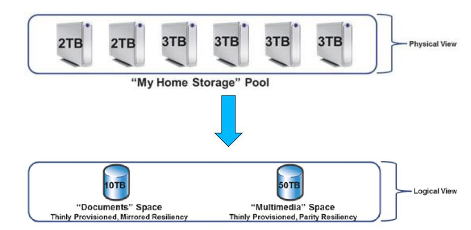
Using the "Storage Spaces" applet in "Windows 8", you create logical "Storage Pools" which are then used to create "Storage Spaces" virtual hard drives. 9
