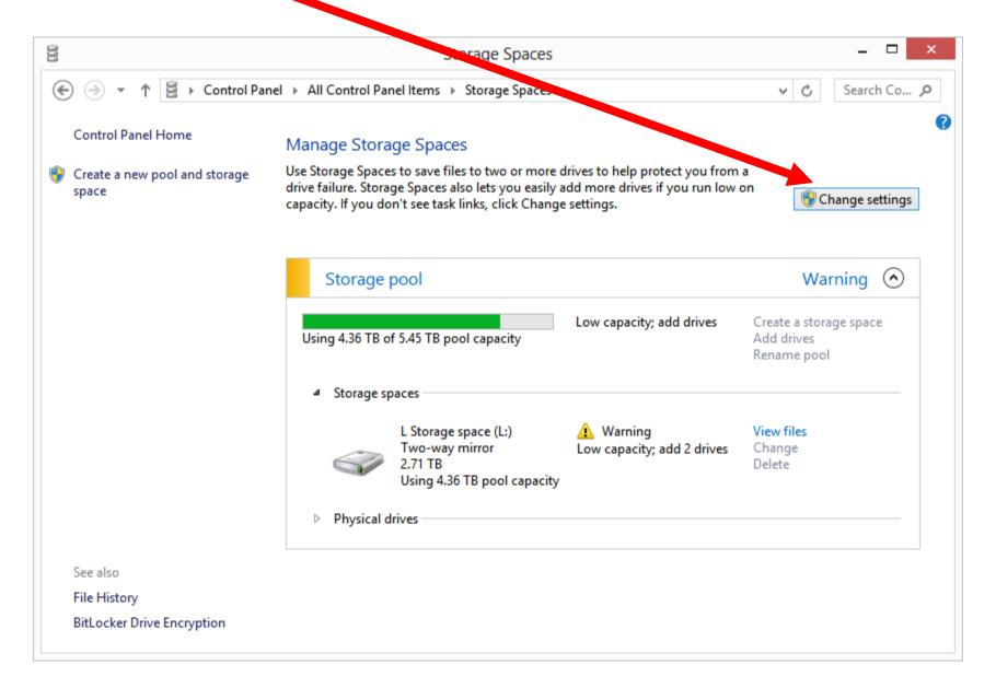
When a physical hard drive in a "Storage Pool" fails or when you physically disconnect the physical hard drive:
