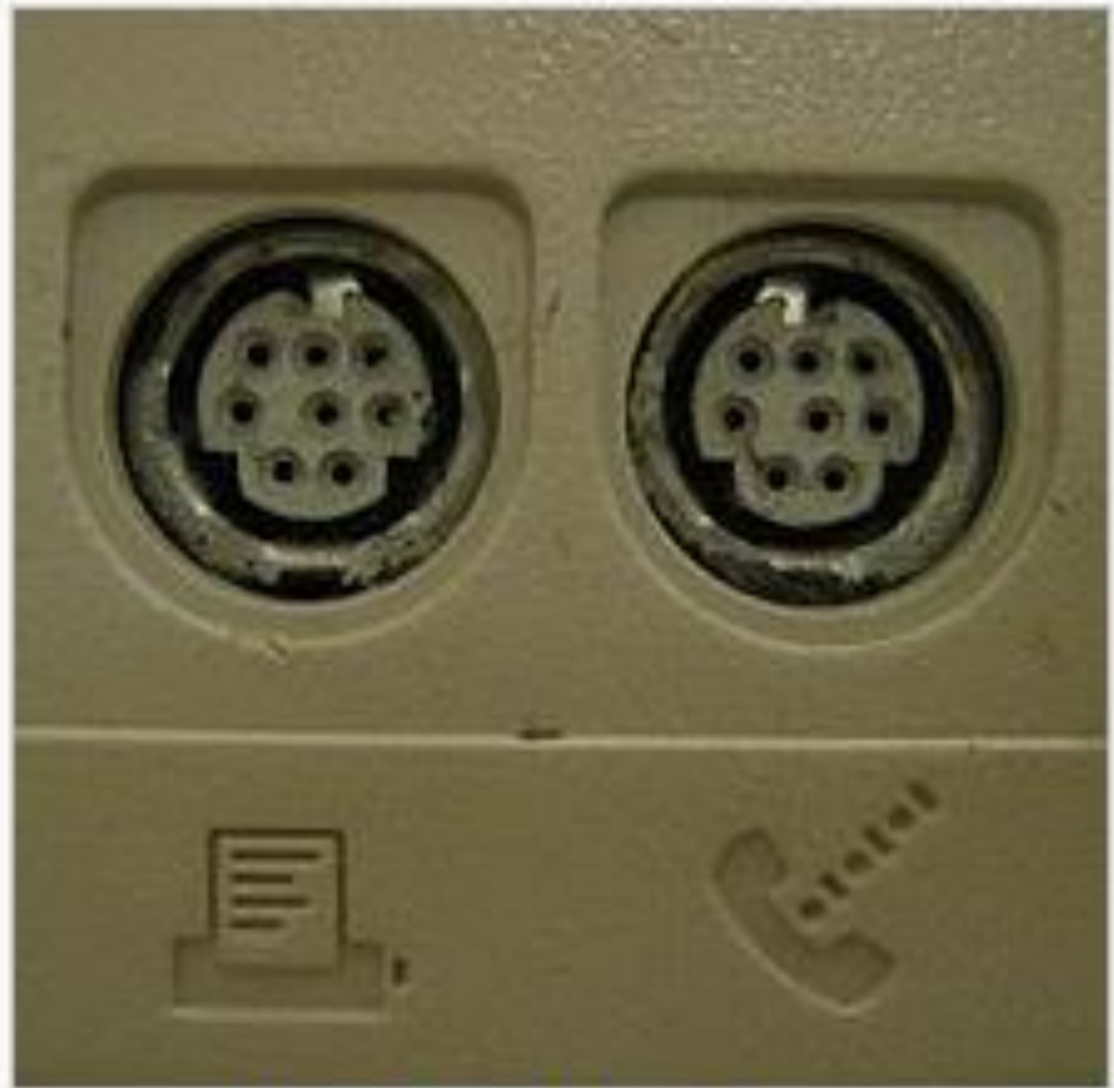
Pair of female Mini DIN-8 connectors used for RS-422 serial ports on a Macintosh LC computer
