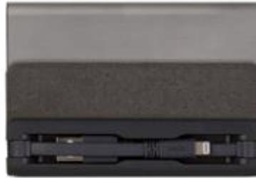
There is a USB socket on one end of the device, which can be used to charge using the cable that came with your smartphone. One advantage of the Ionbank system is that you can use both cables; one will charge your smartphone first then the other will charge the Ionbank.
