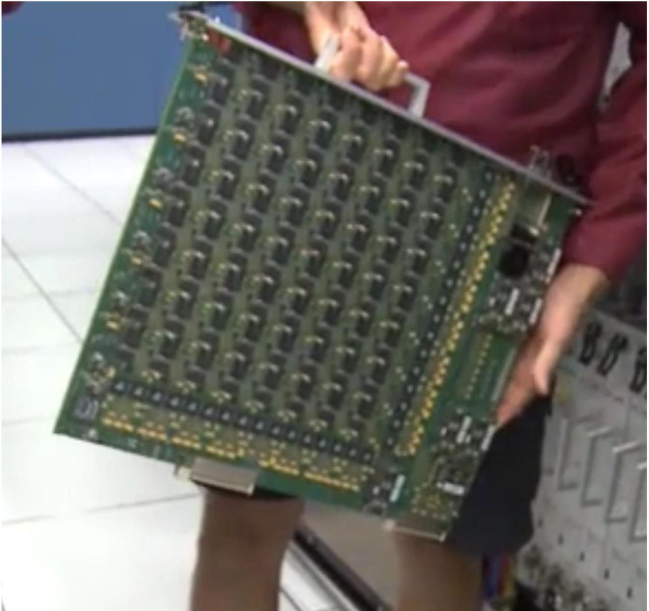
Each of the boards comprising the correlator contains some 180 ICs each with from 250 to 600 pins. VLA personnel state that it is five times faster than the fastest general purpose computer in the world!
